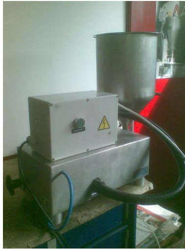
Liquid tube filler 2 – 20 ell.15 – 100 ml.
