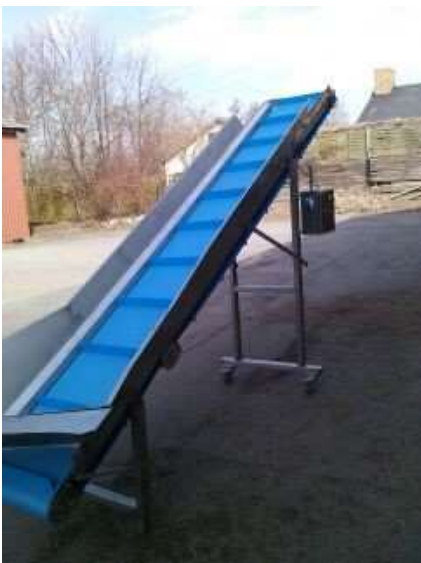
Serviced Belt conveyor 450 x 4000 mm for wet and dry Food Products
