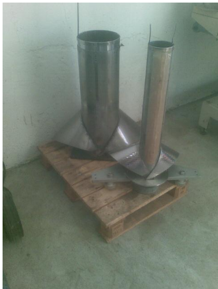
Figur 1 Forming tube for. Hassia-Redatron bagger with hot air vertical sealing
