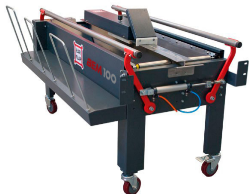
Carton Box Holder for Product infeed... Model BEM 100-PA2 with Pneumatic Box Fix and Push-in Function.
