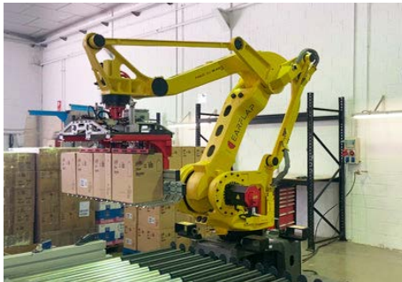
Detergent palletizing Double palletizing station for detergent boxes with quadruple head and automatic pallet feeding.
