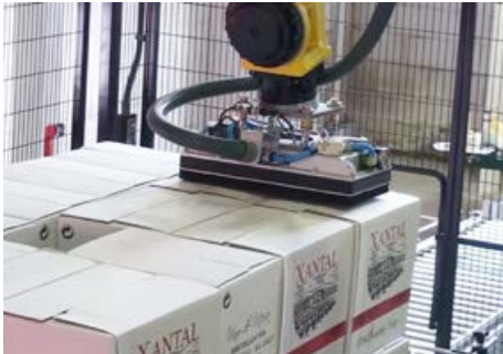
Palletizing boxes with bottles Automatic palletizing cell with robot. The robot supplies the pallets itself, reducing production costs and increasing productivity.
