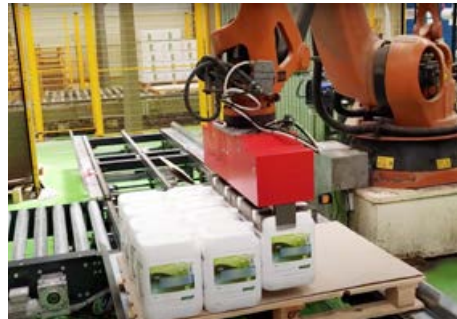
Robot with gripper adapted for palletizing canisters Study, realization and installation of a handling head adapted for palletizing bottles with a handle.
