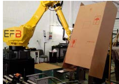
Box forming with robot Special application for the forming of large boxes with an anthropomorphic robot and sealed with a self-adjusting head closer.
