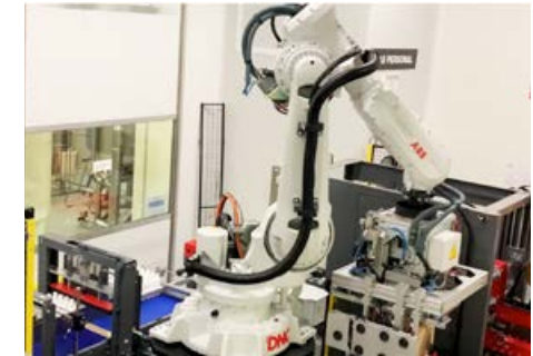
Ultra-compact end-of-line Installation of a single robot that forms the box, fills it with the product and palletizes. Development of multifunction head.
