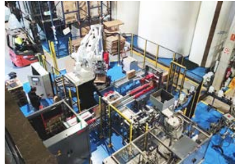
Robotic cell for packing and palletizing bottles with a single robot Automated case erecting, taping, and closing. Project design incorporating necessary aisle and walkway space as per customer requirements.
