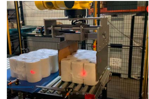
Palletizing and wrapping of paper rolls Automatic cell for palletizing coil packs and annoying pallets up to 3 m high.
